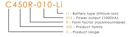
The CertaUPS UPS systems follow a standard part code format always starting with C followed by a number which represents the model. The form factor follows, where an R is present the UPS can be rackmounted or if there is no letter the UPS is tower only.
